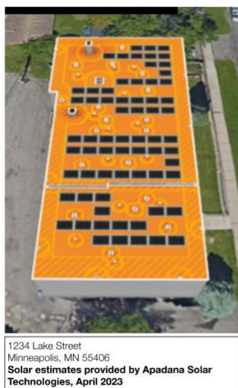
Figure D-7. Example applying Xcel Energy's Solar*Rewards® for Income-Qualified For-Profit for a 27.4 kWdc system. (Image adapted with permission from Apadana Solar Technologies).
